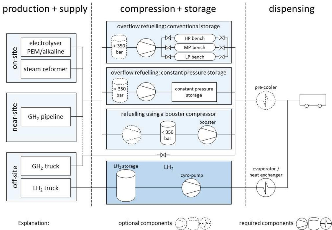
**Figure 2** Scheme of the available main design options for an HRS
